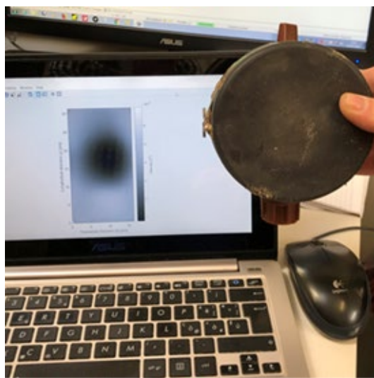
Figure 4: Plastic-cased mine and its HSR image when buried at 30 mm depth in natural soil.
