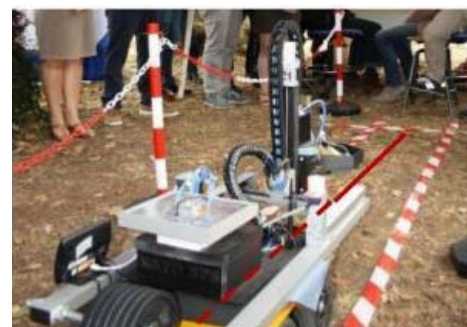
Figure 1 – (Top) Robotic platform in laboratory and a small (11 cm diameter) PMN-4 plastic landmine, (Bottom) demonstration in a field.
