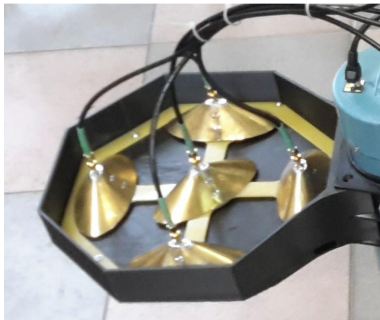
Figure 4. 1Tx+4Rx antenna system for the impulse GPR is shown in the octagonal 3-D printed case.
