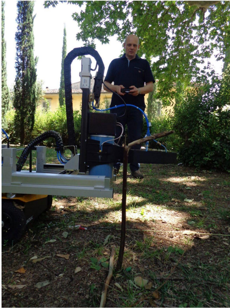
Figure 5. Picture of the robot scanning a lane with width (30 cm) on a natural ground. Three buried targets ( PMN-1 , PMN-4 plastic-cased landmines and a metal tobacco tin) at depth about 5 cm and relative distance about 50 cm.
