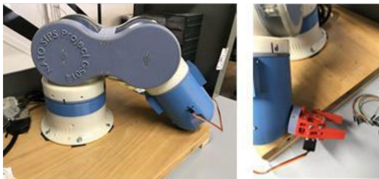
Figure 2. (Left) Articulated robotic arm. (Right) End effector to be used for manipulating a sensorized prodder.
