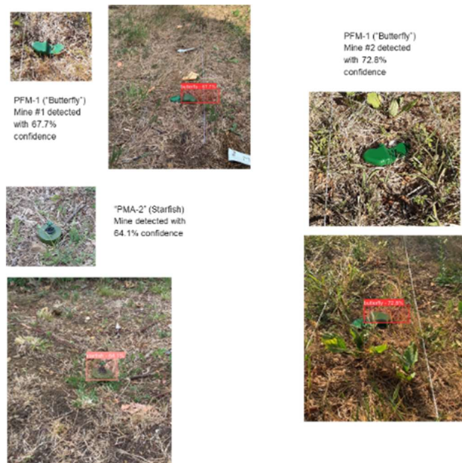
Fig. 3.. Surface threat detection using AI. (See also the video: https://drive.google.com/file/d/1eZaCW97h4hpwm2b-fdL7MBNvrcfdxQpJ/view?usp=drive_link )
