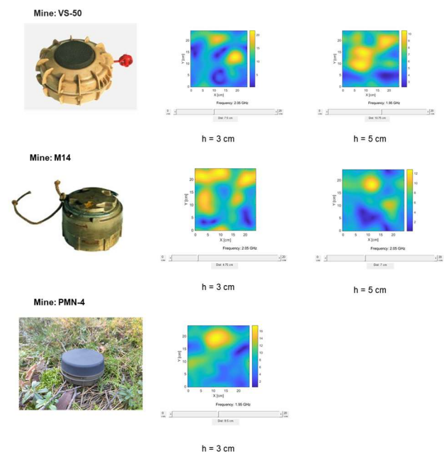
Fig. 5. (Left) picture of the AP landmine; (Centre) Amplitude image of HSR at antenna height h=3 cm and (Right) at h=5 cm.
