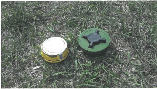
Fig. 4. Target descriptions. (Top) Metal tin of 10 cm diameter and PMN-2 plastic landmine 12 cm diameter.
