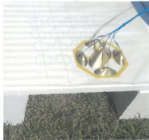
Fig. 5. Outdoor experimental set up. (Top) Grid of 6 \times 5 antenna positions drawn on Styrofoam sheet. (Bottom) Antenna position in the origin of the X–Y coordinate system for the background signal acquisition. Antenna height from the ground is about 30 cm. The receiving antennae RX1 and RX3 are aligned on the OY-axis, while RX2 and RX4 are aligned on the OX-axis.
